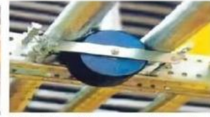
Adjust the sliding speed of goods through the pull rod.
